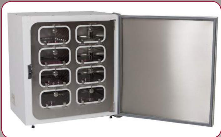
Touch T190S CO<sub>2</sub> incubator with 8 inner glass door option fitted.
